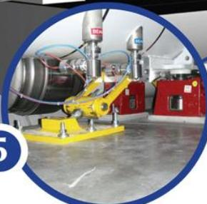
A new longitudinal restraining system is being fitted to 50 quadrupole magnets
