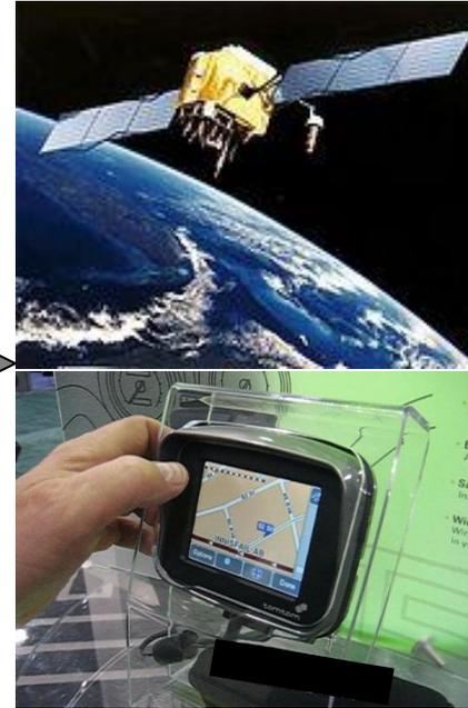
For GPS to work, we have to take into account the correction due to time dilation. Otherwise, there would be a position error of around 10m after just 5 minutes of travel-time!
