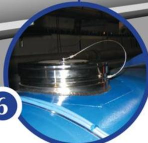
Nearly 900 new helium pressure release ports are being installed around the machine
