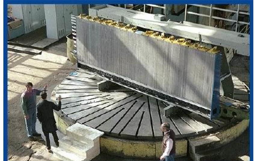
Module assembly (18 submodules each), 64 modules form the TILE barrel
