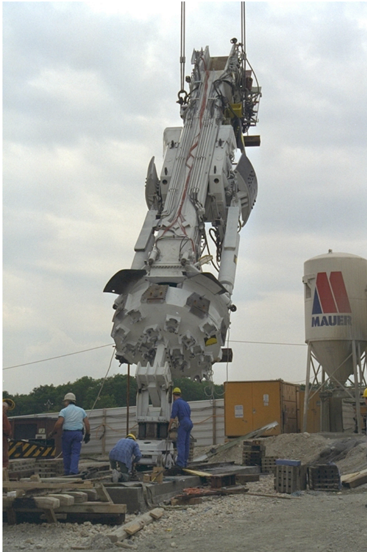
The tunneling machine and early conditions in one of the proton transfer tunnels
