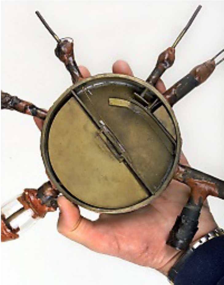
The first cyclotron with a diameter of 5 inches
