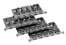
Strain gages, strain-gage-based transducers, thermocouples, LVDTs, potentiometers and other transducers can be intermixed in multiples of 5 by choosing the appropriate sensor card.
