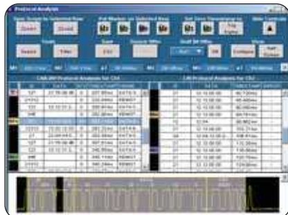
► CAN and LIN Timing and Protocol Decode.
