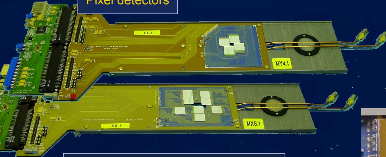
$\sim$  100 pixel detectors (radiation tolerant)
