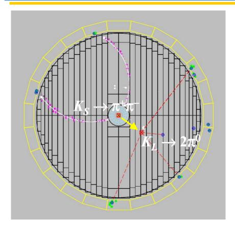
$K_L$  tagged by  $K_S \to \pi^+\pi^-$  vertex at IP Efficiency ~ 70% (mainly geometrical)  $K_L$  angular resolution: ~ 1°
