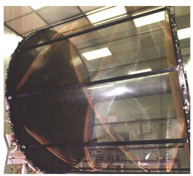
$4m-\varnothing$ , 3.75m—length, all-stereo  $\sigma_p/p = 0.4$  % (tracks with  $\theta > 45^\circ$ )  $\sigma_x^{hit} = 150 \ \mu m \ (xy)$ , 2 mm (z)  $\sigma_x^{vertex} \sim 1 \ mm$
