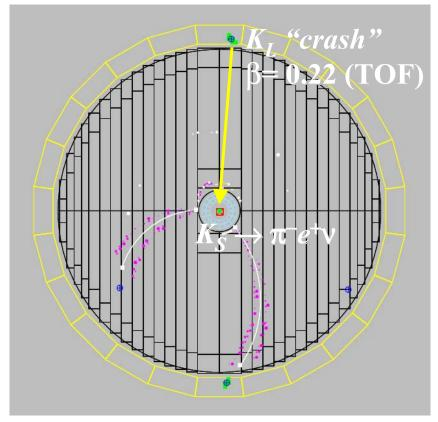
$K_S$  tagged by  $K_L$  interaction in EmC Efficiency ~ 30% (largely geometrical)  $K_S$  angular resolution: ~ 1° (0.3° in  $\phi$ )  $K_S$  momentum resolution: ~ 1 MeV
