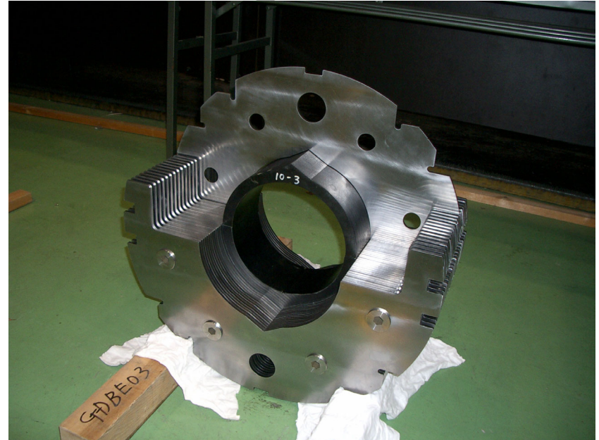
Trial magnet (Plastic collar, Iron yoke)
