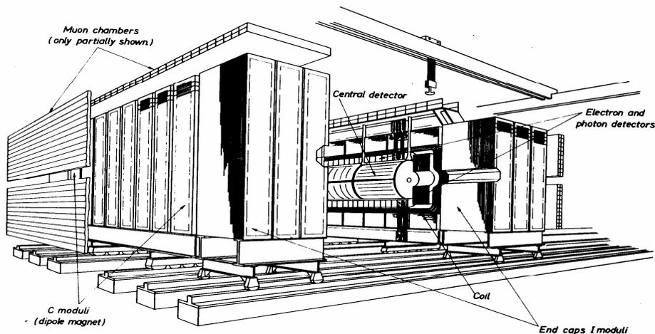
Fig. 1. The Large Angle Detector of the UA1 Apparatus.
