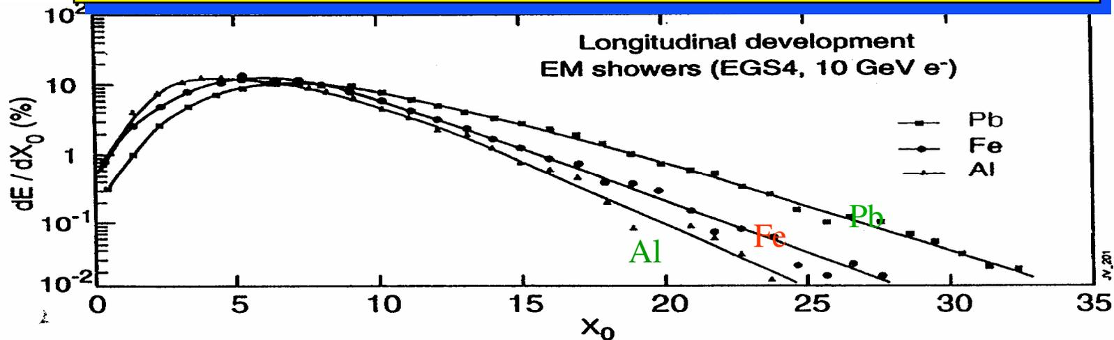
$$t_{\max}(X_0) \sim \ln \frac{E_0}{\epsilon} \pm 0.5 \quad +/- \text{ for } \gamma/e$$
