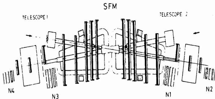
detector as used in the CHOV experiment (R401). N, Neutron detectors. Compensator chambers and Trigger/Monitor hodoscopes are shown by lines.
