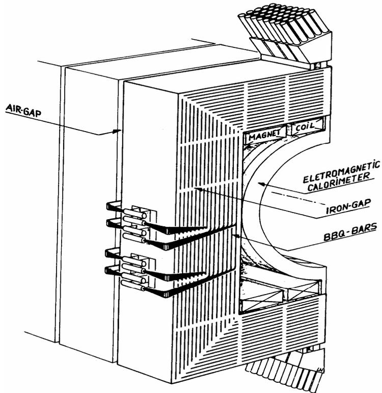
Fig. 2. One of the 16 "C" models comprising the magnet yoke and hadron calorimeter.
