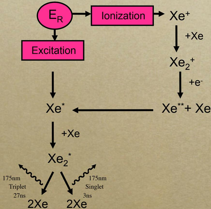
*Nuclear-recoil pulses are faster than electron recoil ones.*
