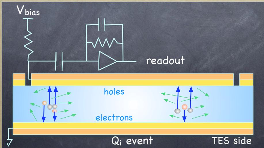
*The particle interaction breaks up the  $e$ -hole pairs in the crystal.*
