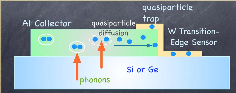
*Phonons propagate to superconducting Al fins where they break cooper pairs.*
