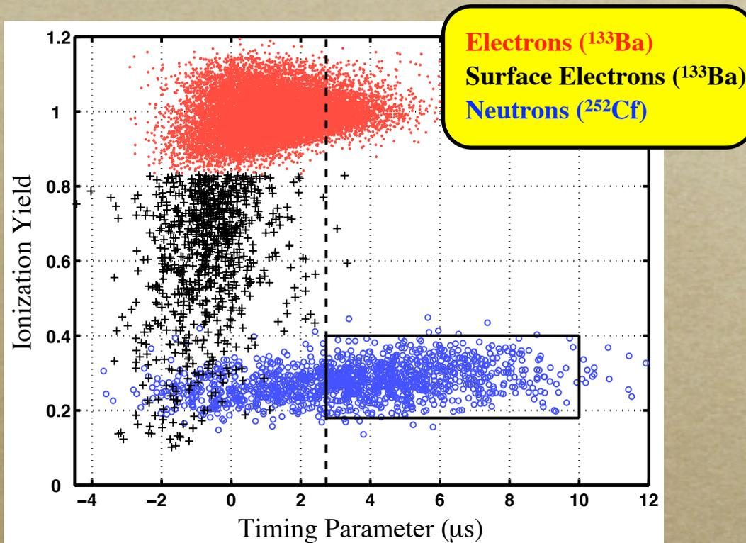
*Events near the crystal's surface produce a different frequency spectrum of phonons.*
