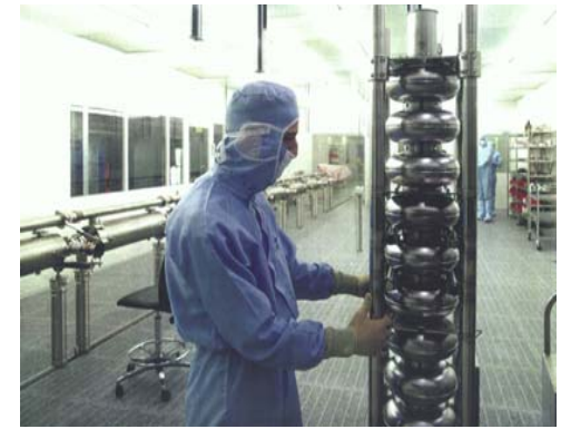
Cleanroom handling of niobium cavities
