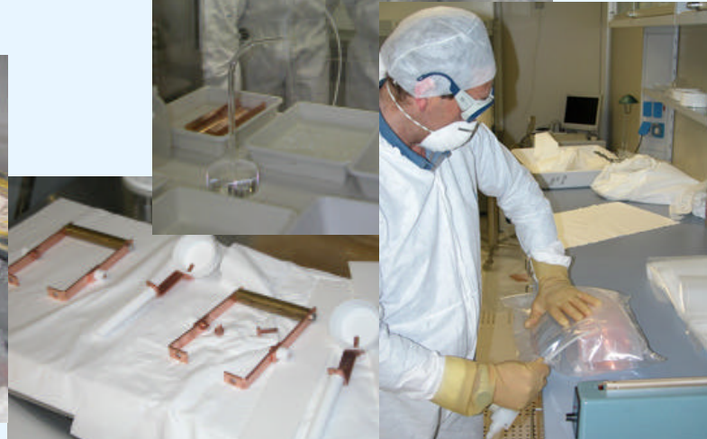
Cu etching with super- and ultra-pure HCl solutions, dried and sealed in HP N 2
