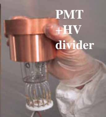
Cu etching with super- and ultra-pure HCl solutions, dried and sealed in HP N 2
