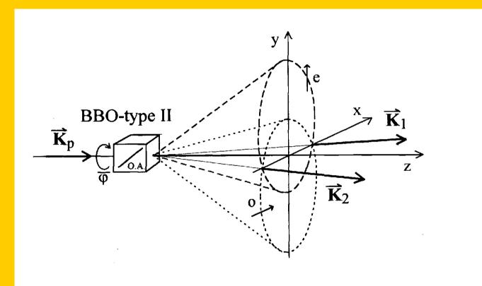
On mode  $K_1$ : field operators  $\hat{a}_1 \equiv \hat{a}_{1\perp}, \hat{b}_1 \equiv \hat{a}_{1\perp}$ On mode  $K_2$ : field operators  $\hat{a}_2 \equiv \hat{a}_{2\perp}, \hat{b}_2 \equiv \hat{a}_{2\perp}$
