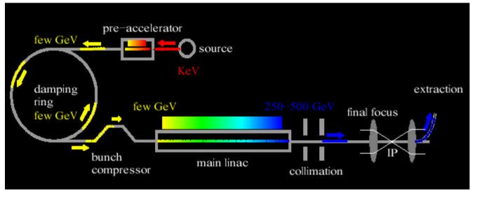
For E > 200 GeV need to build linear colliders
