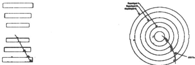
$\pi^+$  then ranges out in an Range Stack (scint. + straw ch.)
