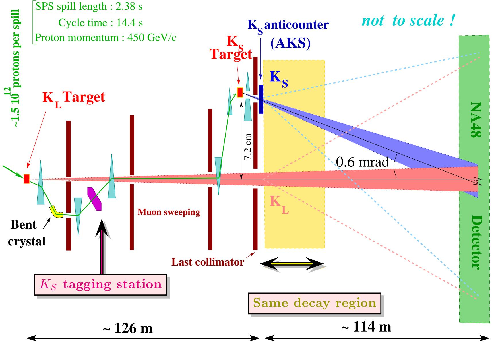
$K_S$  and  $K_L$  beams are distinguished by proton tagging upstream of the  $K_S$  target
