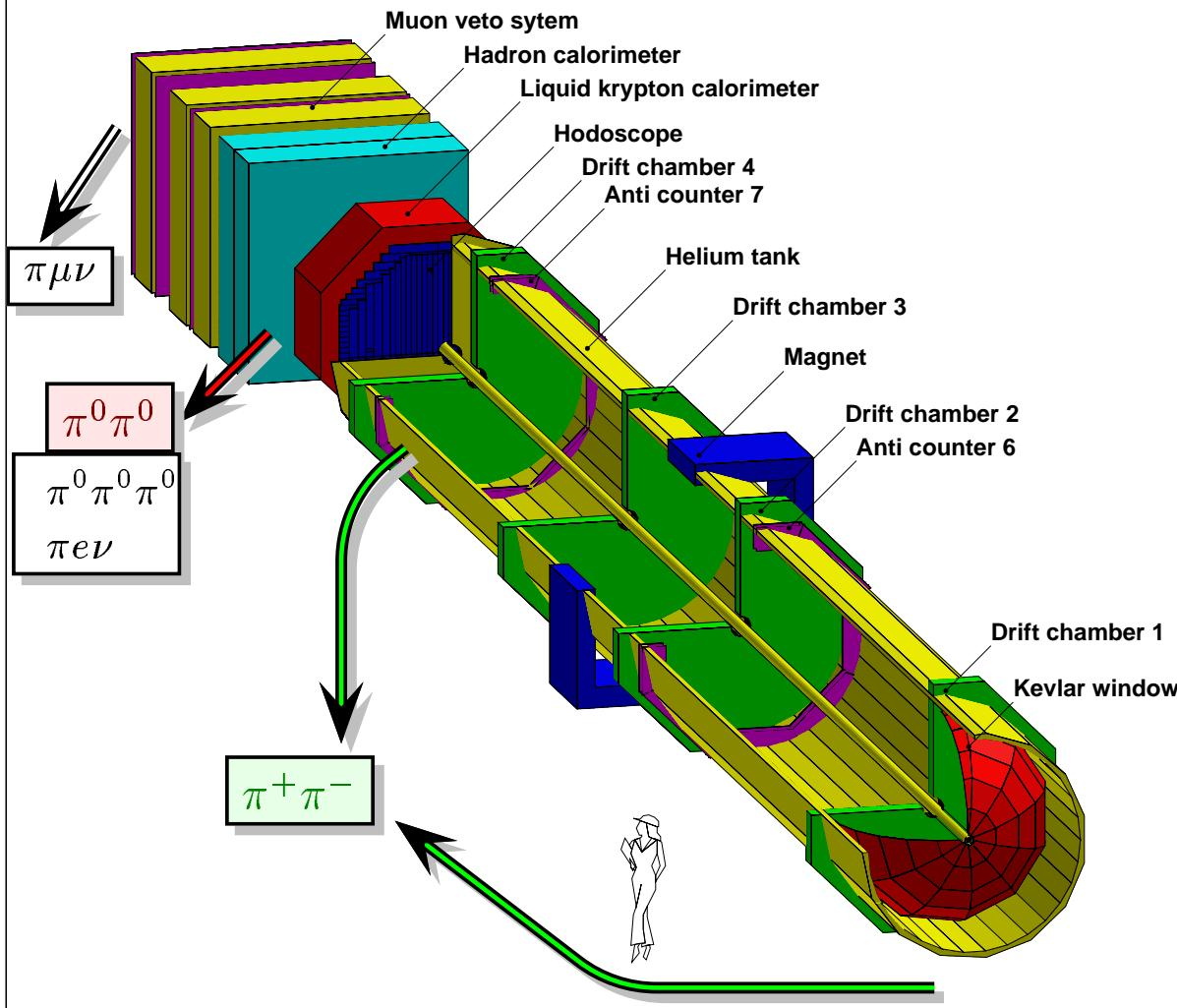
High resolution detector to identify  $\pi^+\pi^-$  and  $\pi^0\pi^0$  and 3-body background
