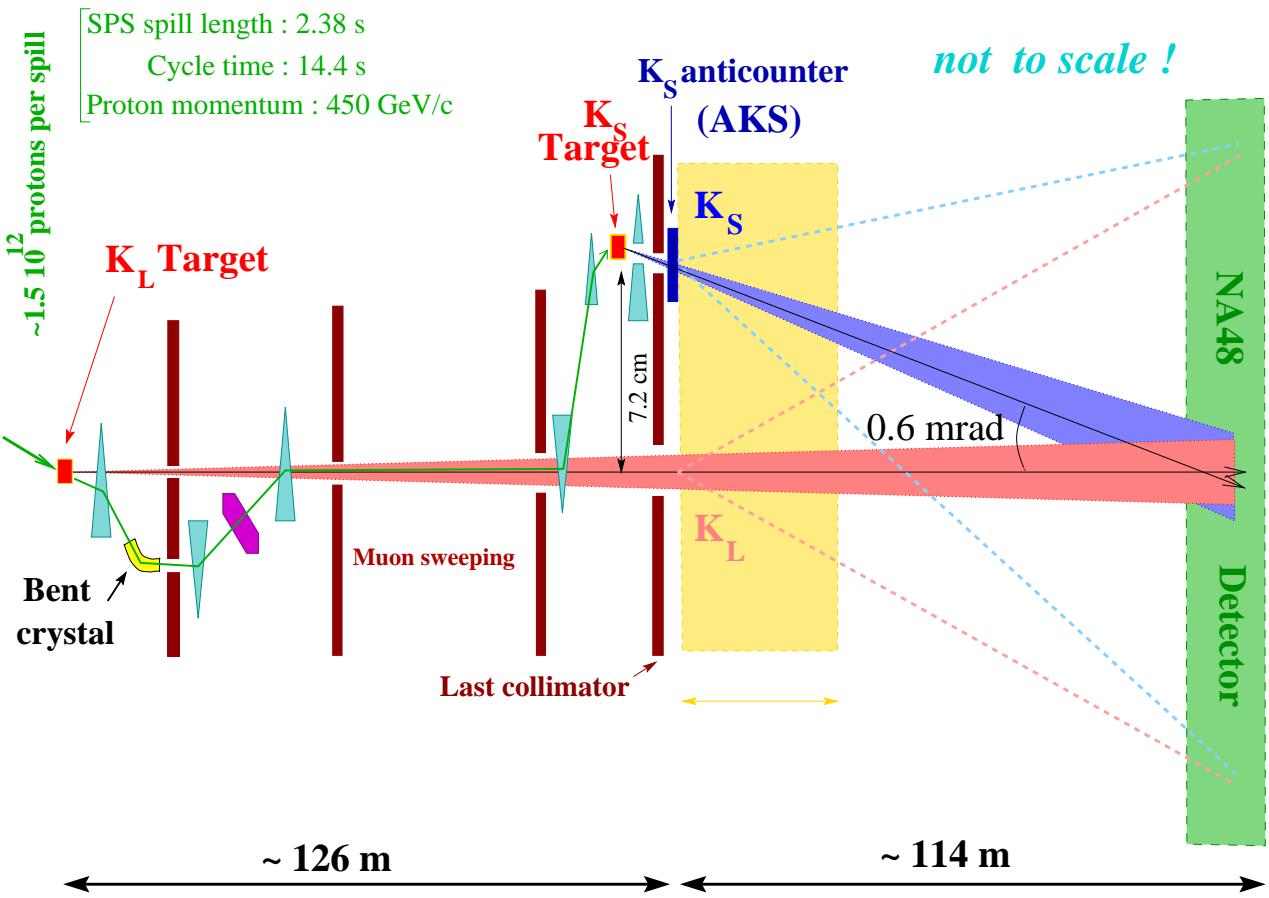
Decay region is defined by applying cuts on the reconstructed kaon energy and the decay vertex position (and AKS for the beginning of the  $K_S$  decays)
