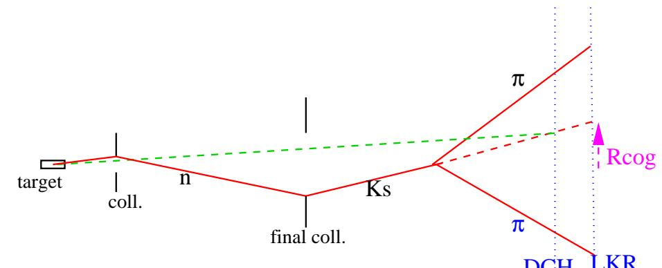
Background from beam scattering produces  $K_S$  in final collimator
