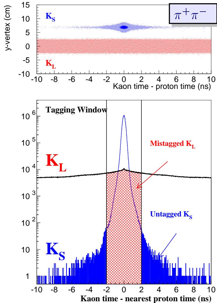
→ in both decay modes  $K_S$  tagged by comparing the event time to proton times as they pass through tagging station
